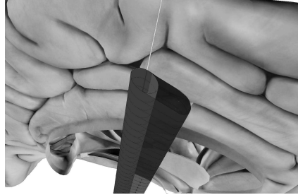
Figure 6. Close-up in the 3D representation of the physics-based risk volume (darker shape), compared to the geometry-based safety margin (cylinder).
