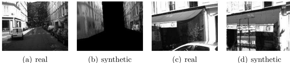
Figure 11: Two cases where the proposed method fails. (a-b) the 3D scene texture quality is extremely poor, particularly on the left. (c-d) a combination of partial occultation, erroneous texture mapping and parallax of ban, which is in 3D in reality but mapped to the vertical plane of a building in the 3D virtual scene.
