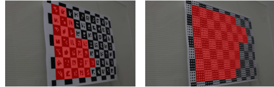
Figure 9: Detected squares in CALTag vs. BlurTag. Left: Detected squares of CALTag-based checkerboard. Right: Result of BlurTag-based checkerboard.
