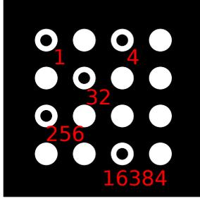
Figure 3: Sample code with active bits  $2^0$ ,  $2^2$ ,  $2^5$ ,  $2^8$  and  $2^{14}$  leading to the ID 16677. The bits are using a lexicographical order. Codes are unique under rotation and mirroring.
