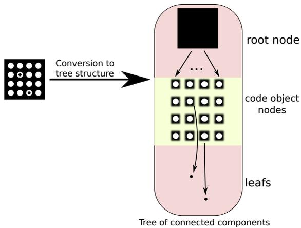
Figure 6: Conversion from pattern to tree structure. The hierarchy of the connected components is encoded as parent/children relations in the tree.
