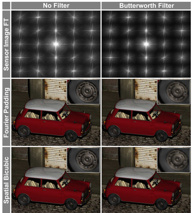
Fig. 9 Analyzing aliasing artifacts. Multiplexing a light field with 5 \times 5 views onto a sensor is simulated without (left column) and with (right column) a synthetic optical anti-aliasing filter applied. The Fourier tiles of the sensor image slightly overlap without any filtering (upper left). A proper anti-aliasing filter mitigates this overlap and thereby artifacts in the reconstructions (right). A spatial processing of multiplexed data (lower left) is usually more robust to signal aliasing than a corresponding Fourier approach (center left).
