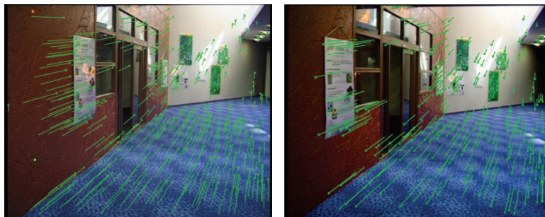
Figure 12. Corridor, epipolar constraint. The AC method (left) retrieves 423 correspondences. Of these, 405 correspondences have rank 1, 13 rank 2, 2 rank 3, 1 rank 4, 1 rank 6, and 1 rank 10. The NN-T+O method (right) retrieves 295 out of 316 NN-T matches. The additional correspondences are on the carpet and on the wall. 1,269 keypoints were extracted from image 1 and 1,360 from image 2.
