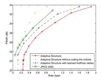
Fig. 7. Rate-distortion curves for K=256 with blocks 8x8
