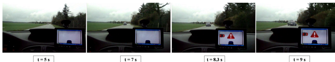
Figure 10: Dangerous situation detected during the field trials (view from inside the Priority Vehicle).
