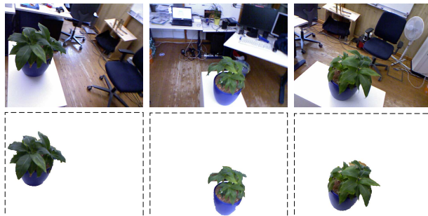
Figure 1. Multi-view object segmentation (MVOS) using our method with the 3 wide-baseline views shown only, with no photo-consistency hypothesis and no user interaction.
