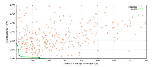
Figure 8: Pareto front for the resistance and the deadweight-deviation criteria
