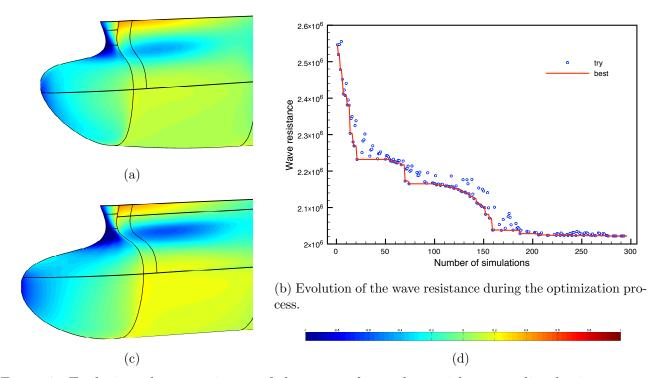
Figure 7: Evolution of wave-resistance & bow-area shape along with source distribution
