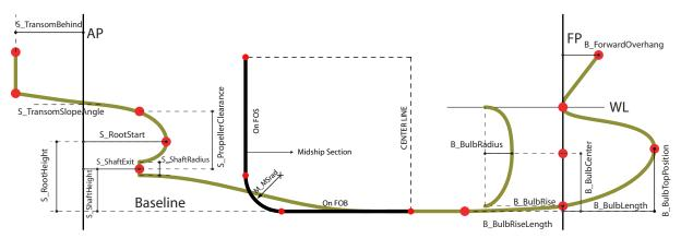
Figure 2: Exposed parameters for aft and bow parts of the ship and midship section
