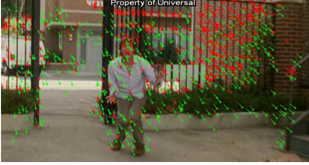
Figure 2. Visualization of inlier matches of the robustly estimated homography. Green arrows correspond to SURF descriptor matches, and red ones to dense optical flow.
