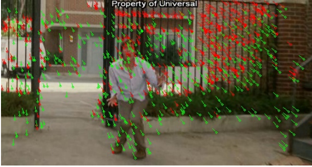
Figure 2. Visualization of inlier matches of the robustly estimated homography. Green arrows correspond to SURF descriptor matches, and red ones to dense optical flow.
