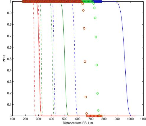
Fig. 5. PDR as function of the receiving vehicular. Solid line  $\alpha = 2$ , dashed line  $\alpha = 3$ , dashed-dotted line  $\alpha = 4$ . Blue - 3 cars/km, green - 25 cars/km, red - 80 cars/km. Circles correspond to evaluation based on the experimental data as described in Section II.
