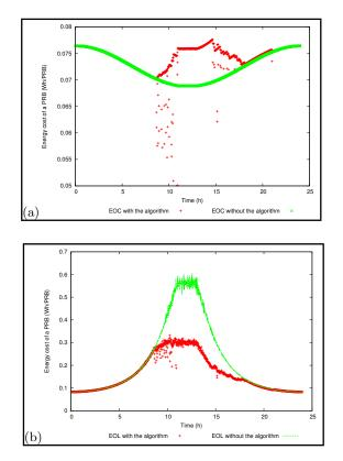
Figure 10: Energy cost of an offered PRB (a) and a used one (b)
