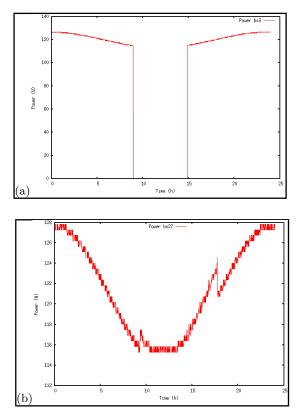
Figure 9: Power consumption of switched off eNodeB (a) and absorbing traffic one (b)
