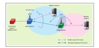
Figure 1: LTE relay network architecture
