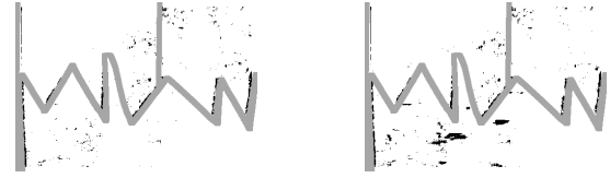
Figure 3. Bad pixels ( \delta = 1 ) using ENCC (left) and NCC (right) without sub-pixel refinement (Shaded area contains occlusions and depth discontinuities).
