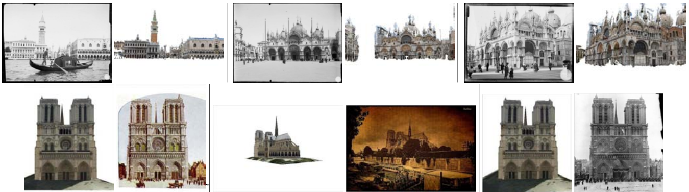
Fig. 11. Alignment of historical photographs of San Marco’s Square (top) and Notre Dame of Paris (bottom) to their respective 3D models.
