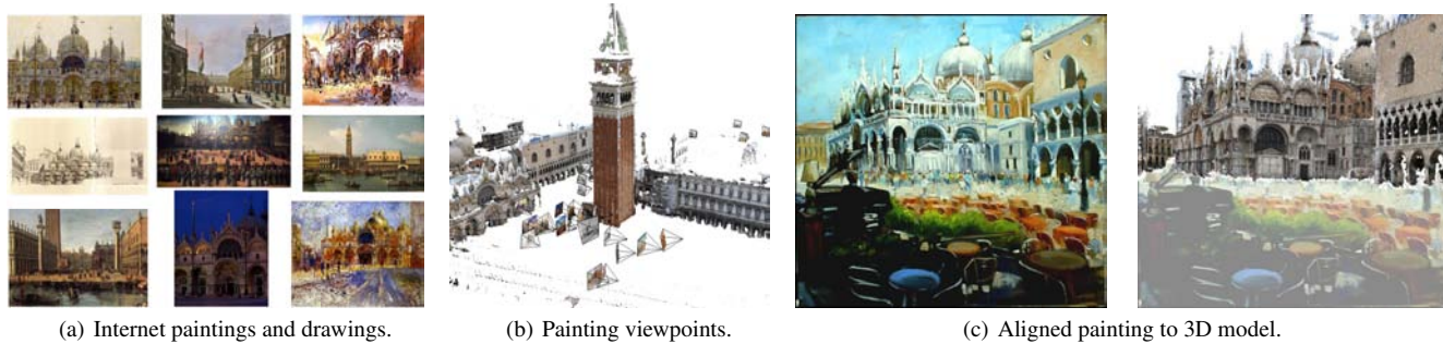
Fig. 1. Our system automatically aligns and recovers the viewpoint of paintings, drawings, and historical photographs to a 3D model of an architectural site.
