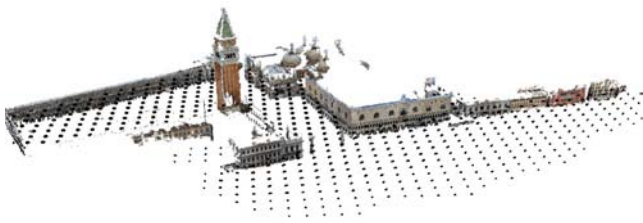
Fig. 3. Example sampled viewpoints. Camera positions are sampled on the ground plane on a regular 100 \times 100 grid. 24 camera orientations are used for each viewpoint. Cameras not viewing any portion of the 3D model are discarded. This procedure results in about 45,000 valid views for the depicted 3D model.
