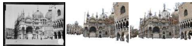
Fig. 10. ICP-like fine alignment for perspective correct scene depictions. Given the coarse alignment, at each iteration we find a dense set of inlier correspondences with RANSAC for HOG features computed over a grid. We then update the viewpoint and iterate. Notice that the fine alignment step produces a tighter, more accurate fit.
