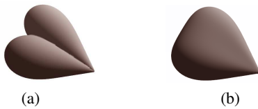
Figure 20: The positioning of two scale-invariant primitives in a "V" shape illustrates the good behavior of the SCALIS blending, which is the same at both extremities of the shape (we can note that the thin extremity is not blurred). (a) blending with a "max", (b) blending with a "+".
