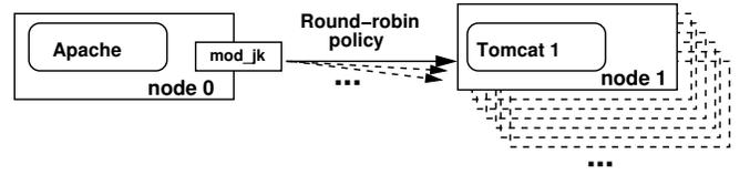
Fig. 7: Architecture of the replicated web-server system
