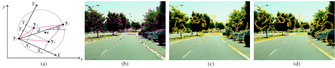
Fig. 3: (a) Geometry hashing via the quad structure and (b) a query frame with its extracted Harris points. (c) The valid quads of the query and (d) the reference corresponding frame; red dots denote the centroids of the quads.
