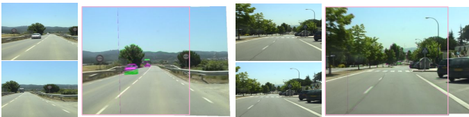
Fig. 12: Alignment of partially overlapped sequences. Input, retrieved and aligned frames by the Quad-Tree algorithm for the (left) Backroad and (right) Campus sequence with 50% and 70% overlap ratio respectively; the pink window marks the input frame.
