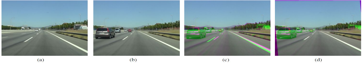
Fig. 7: An example of the proposed method for the Highway dataset. (a) A query frame and (b) the retrieved frame with the best score. The space-time alignment after (c) 1 and (d) 10 iterations. Differences between query and reference frame are illustrated using lawn-green and hot-pink colors.
