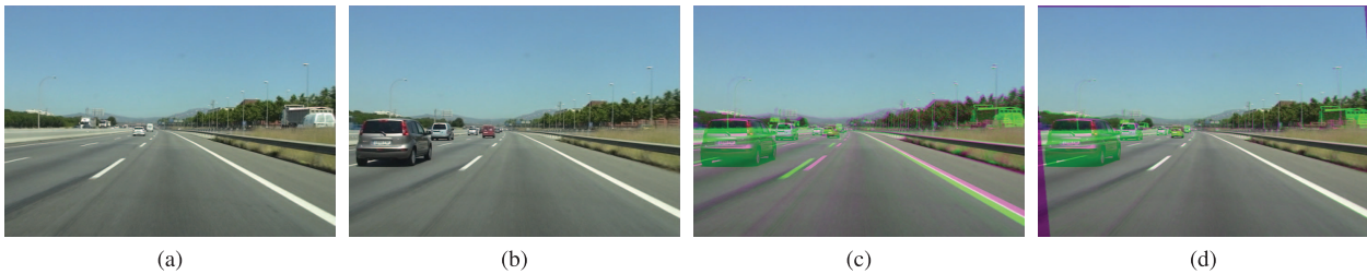
Fig. 7. An example of the proposed method for the Highway data set. (a) A query frame and (b) the retrieved frame with the best score. The space-time alignment after (c) 1 and (d) 10 iterations. Differences between query and reference frame are illustrated using lawn-green and hot-pink colors.
