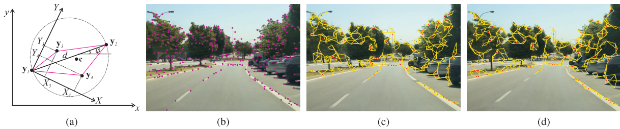
Fig. 3. (a) Geometry hashing via the quad structure and (b) a query frame with its extracted Harris points. (c) The valid quads of the query and (d) the reference corresponding frame; red dots denote the centroids of the quads.
