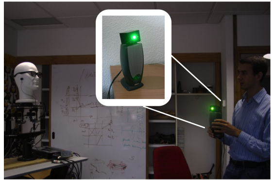
Fig. 2. Audio-visual device used to align the auditory and visual spaces. An LED light bulb is mounted onto a speaker which makes the visual localization more precise. White noise is played throughout the recording to improve the auditory localization.
