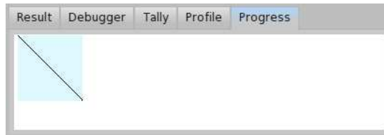
Figure 18.22: Progress of Petit Parser that parses input in linear amount of steps.
