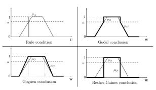
Fig. 2. Inference with one gradual rule and a precise input
