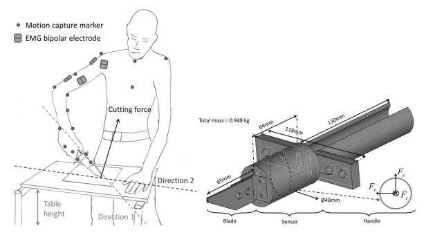
**Figure 1:** Experimental situation showing the instrumented knife, bipolar EMG electrodes, and the active markers for the assessments of the cutting forces and movement in 3D. Motion capture markers were placed on standard anatomical landmarks. The resulting cutting force was measured mainly in the (y,z) plane, and lateral bending effects appeared in the x direction.
