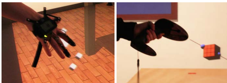
Figure 2: Left: Visual representation of the palm and three fingertips in the VE (cubes are shown away from the fingers for clarity of illustration). Right: Wand selection used for comparison.
