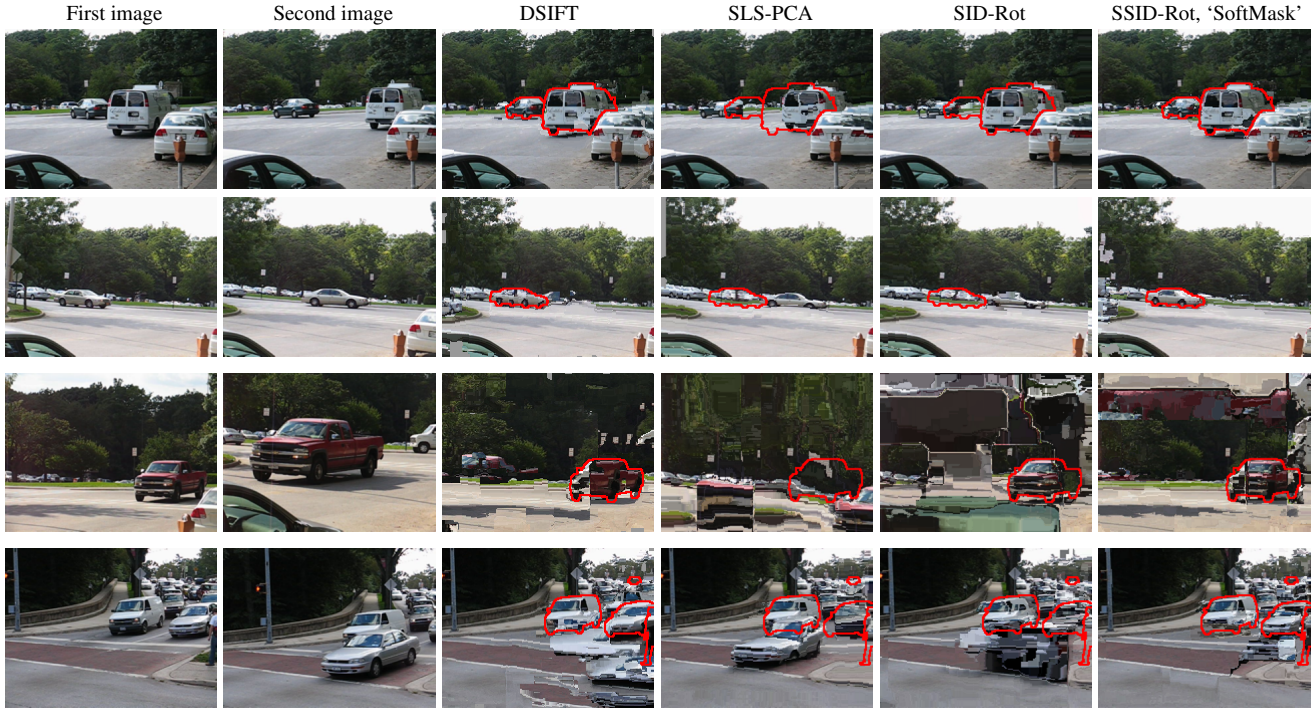
Figure 5. Large displacement image matching using SIFT flow, for different considered in this paper. We warp image 2 to image 1 using SIFT-Flow with different descriptors. The ground truth segmentation masks of image 1 are overlaid in red (a good registration should bring the object in alignment with the segmentation mask). We observe that segmentation-aware variant SSID-Rot does best, and is better than SID-Rot (please zoom in for details). Similar improvements were observed for SDSIFT over DSIFT.
