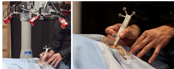
Figure 13: Overview of our setup: mannequin and microscope where 6 infrared cameras are attached. These cameras allow to track in real-time the motion of the surgical tools.
