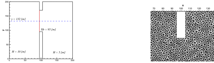
Figure 5: Asymmetric dam break. Left: computational domain. Right: mesh close up ( h \approx 2 )
