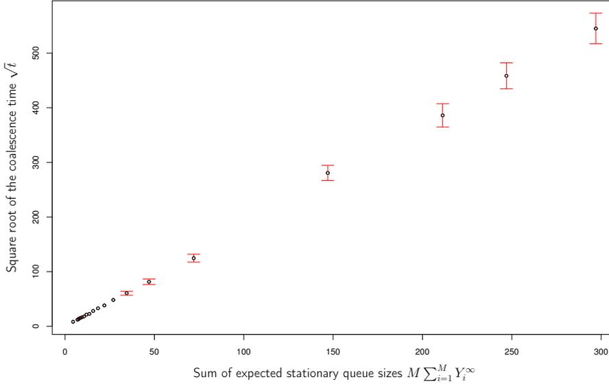
Figure 6: Asymptotic behavior of (the square root of) the coalescence time (number of steps) of our PSA-BP algorithm as the expected queue size grows (increasing with load  $\rho$ ). Notice that due to the doubling period artefact, the observed number of steps is at most twice the actual coalescence time of the simulated trajectories. Circular networks with  $M=3$  queues, capacity  $C = 500$ ,  $\mu = 1$ ,  $p_{i0} = 0.5$ .
