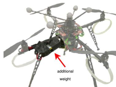
Fig. 4. mikrokopter with the unknown weight attached
