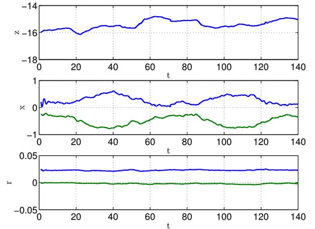
Fig. 8. Time history of the parameters for the case d). Top: parameter  $\gamma_z$ , center: parameter  $\tilde{\gamma}_{xy}$ , bottom: parameter  $r_C$ . It can be noticed that the center of mass estimation is coherent with the rough estimate done
