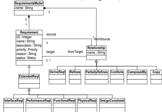
Figure 10 Specialized Requirements Metamodel for SysML Requirements
