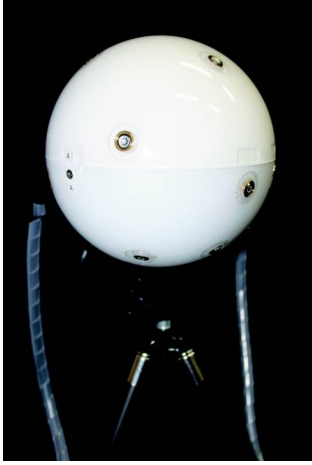
Fig. 2. Fabricated 12-element spherical microphone array of diameter 15 cm. The microphones are mounted on a rigid spherical shell.
