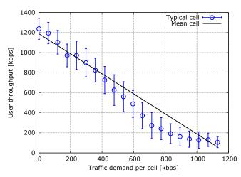
Fig. 4. Mean user throughput in the network versus traffic demand per cell in the full interference model.
