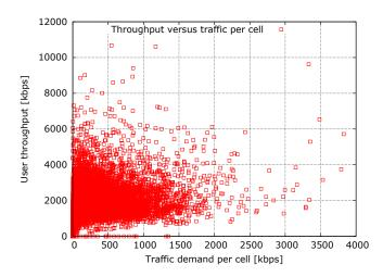
Fig. 1. Local user throughput versus local traffic demand for an operational cellular network. Different points correspond to the measurements made by different cells during different day hours.
