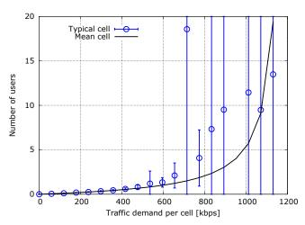
Fig. 3. Number of users per cell versus traffic demand per cell in the full interference model.
