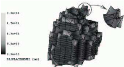
Figure 3. geometry after applying a uniform pressure simulation
