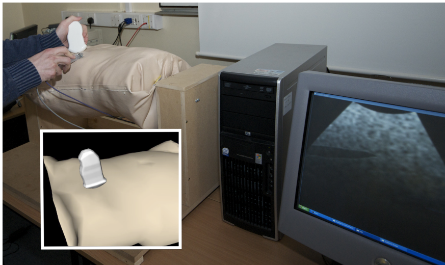
Fig. 7 Mannequin ribcage synchronised with the virtual environment (3D meshes and ultrasound rendering). Inset: patient and ultrasound probe in the virtual environment
