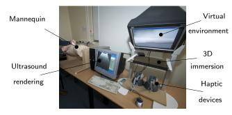
Fig. 8 Integration of Workstation 1 and Workstation 2
