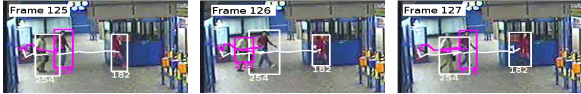
Figure 4. Illustration of the output of the controlled tracking process. Different IDs represent different tracked objects.
