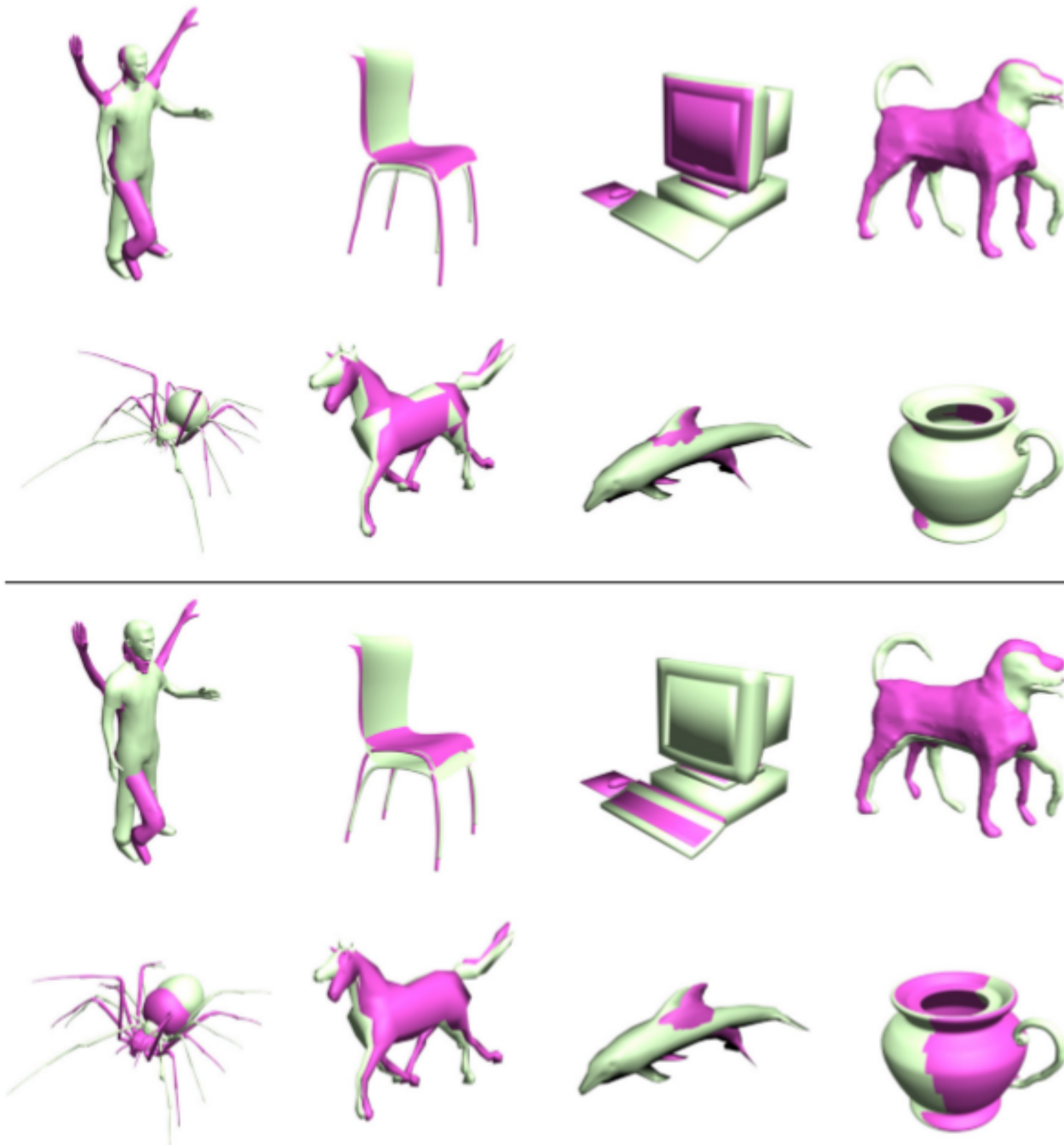
Fig. 9. Comparison of translation and scale normalization using OCSVM (top row) against using the centroid and average distance of the surface (bottom row).
