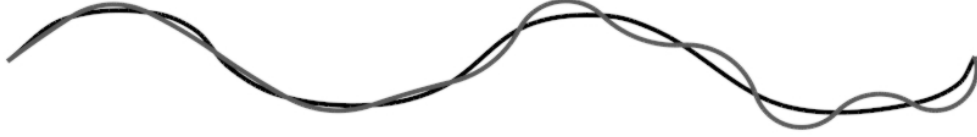
Figure 2: Approximation of a 2d spline (in black) by a polycircle (in grey) with 13 circular arcs. As only points and the first (left) tangent are interpolated, an increasing drift of the approximation can be observed from left to right.
