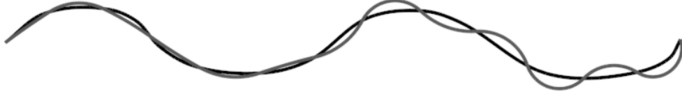
Figure 2: Approximation of a 2d spline (in black) by a polycircle (in grey) with 13 circular arcs. As only points and the first (left) tangent are interpolated, an increasing drift of the approximation can be observed from left to right.
