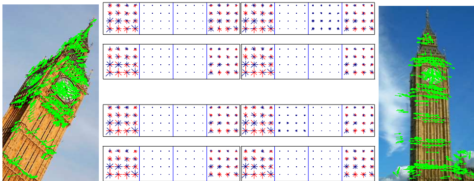
Figure 2: Illustration of the pooling scheme. Hessian-Affine features from each image have been quantized with four visual words and pooled in 8 orientations. Four sub-vectors of CVLAD (top two rows) from image on the left correspondingly match to four CVLAD sub-vectors from image on the right (bottom two rows). Their similarities are (in clockwise): 0.94 , 0.89 , 0.83 and 0.85 . Positive and negative components are colored in red and blue respectively.
