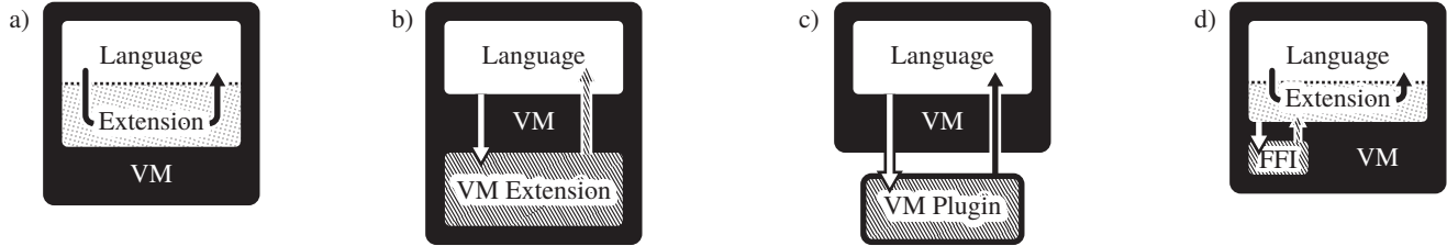
Figure 1: Comparing different extension mechanisms: a) library implemented completely at language-side running on a standard VM, b) language using features from a VM extension, c) language using features from a VM plugin, d) language-side implementation of an extension.
