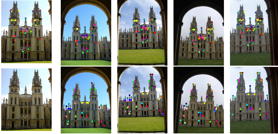
Figure 4: Sample reliable images and features assigned to reliable visual words, when geometry is not used. Left : Query image. Top : Features assigned to reliable visual words that appear in the query image. Bottom : Features in the set of augmented visual words. Note: we only show a subsample of the actual reliable visual words. Each color represents a distinct visual word.
