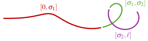
Figure 5: Visual representation of our piecewise summation algorithm applied to the rod's kinematics (one clothoidal element). The length of each subinterval which guarantees a safe evaluation of the geometry is automatically provided by our method.
