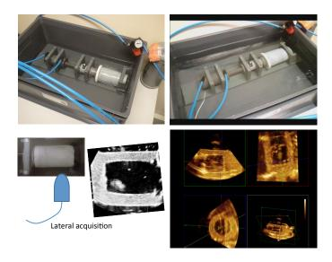
**Fig. 3.** Physical phantom setup. Top: The PVA phantom is placed in a water-filled aquarium. The pneumatic mechanical part is MR compatible and can dissociate or combine compression and rotation. Bottom left: images were acquired from a lateral position of the probe. Bottom right: obtained 3D US image.
