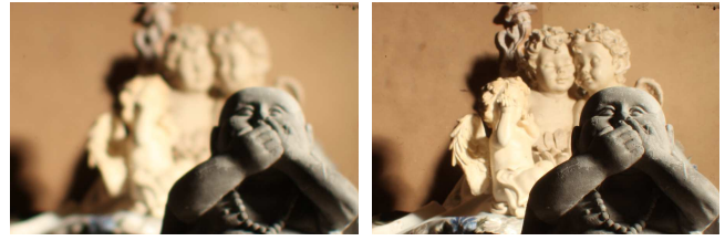
Figure 6: The aperture of the pickup system determines the depth of field of the light-field views (shown is the center view, but other views behave similarly). With and open pickup aperture, depth of field effects can be clearly observed (left). With a closed pickup aperture, the views are sharply imaged over the full depth range (right).
