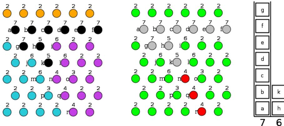
Treatment of priority 6 queue. Tokens (i), (j) (l) and (m) are extracted in this order. (i) is labelled (purple label) and, being labelled "RG LABELLED", it pushes on the HQ tokens (h) and (k). The priority 5 queue being disappeared, (h) and (k) are placed on the current queue.
