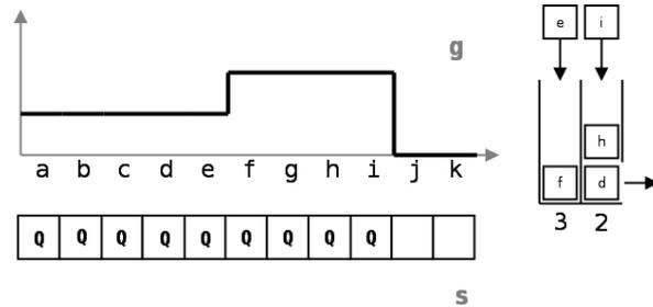
Next step: tokens (d) and (h) are extracted. Token (d) sends (e) on the queue. (h) pushes (i) on the current priority queue. So (i) is processed and pushes (j). The process ends up when (f), (j) and (k) are processed.
