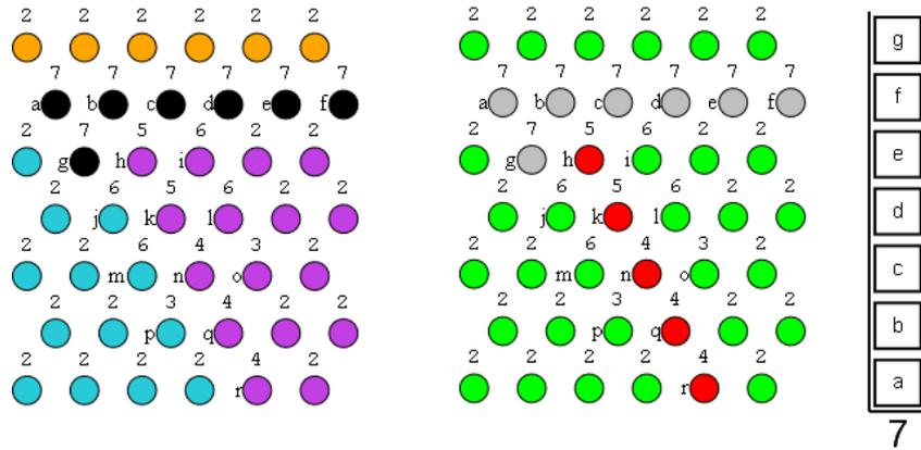
(h) and (k) are extracted from the queue and labelled as WTS points. The rest of the process is similar and will produce the same result as above.
