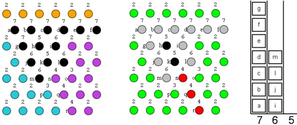
Treatment of priority 4 queue. Tokens (q) (r) and (n) are extracted from the queue. They become WTS points. However, although (n) has point (k) as a candidate, it is not included in the HQ because point (n) is not a point marked "RG LABELLED" (it is not flooded). The queue processing ends (no points are inserted). The priority 5 queue is empty, the process continues with the priority 6 queue.
