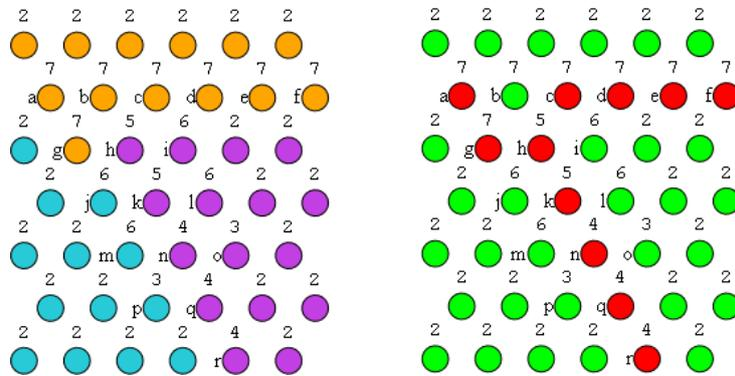
Processing the last queue (priority 7). Points (a), (c), (d), (e) and (f) become WTS points. Point (b) has only two types of neighbors: WTS points and a single labelled point. It takes the label of this latter point (orange label). Note that the final result is different from the result expected above. It is however fully valid. The difference comes from the fact that points have not been processed in the same order in the HQ.
