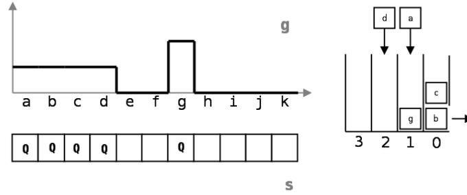
First step of the process: token (b) is extracted, its only CANDIDATE neighbor (a) takes the same label in g, is pushed on the HQ (priority 1) and is tagged QUEUED in s. Same treatment is applied to token (c). Priority 0 queue is then empty and is removed.
