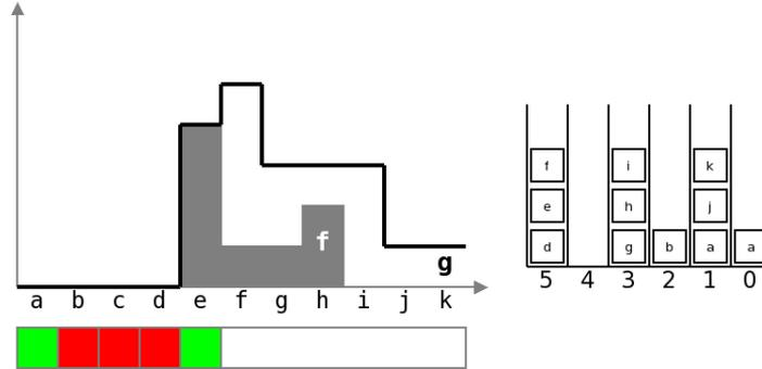
Token (b) exits from the queue, it is marked "FINAL". Point (a), "CANDIDATE" neighbor of (b) takes the value  $\max(g(b), f(a)) = 0$  and is inserted into the priority queue 0. It is marked "QUEUED" in the label image. Same treatment is applied for point (d), marked "FINAL" that pushes point (e) on the stack (marked "QUEUED") with priority  $g(e) = \max(g(d), f(e)) = 4$ .
