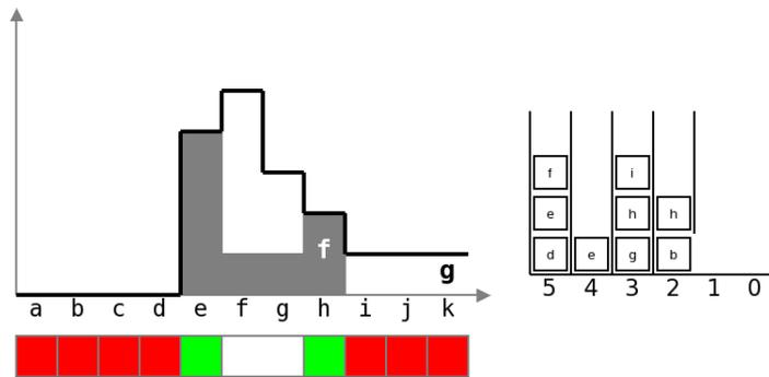
Token (k) is extracted. This token was inserted in the initialisation phase, but it does not matter. We can already guess that the second token corresponding to (k) and located in the same queue will simply be removed when its turn comes. (k) is marked "FINAL" and has no "CANDIDATE" neighbors. Point (i) is also marked "FINAL" and pushes its "CANDIDATE" neighbor (h) on the priority 2 ((h) is marked "QUEUED").  $g(h)$  takes the value 2. The second occurrence of (k) is simply removed.
