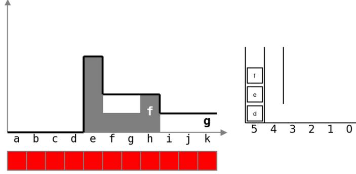
End of the process. Tokens (g), (h) and (i) are extracted. (e) is marked "FINAL". Finally, (d), (e) and (f) are removed from the priority queue 5.
