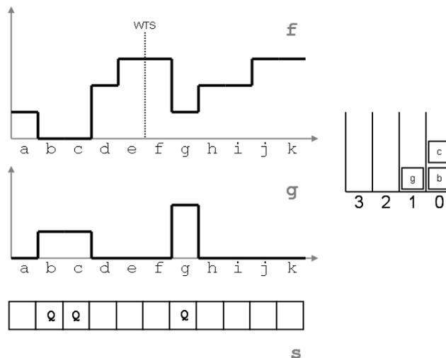
*Initial state: in this example, the flooding sources correspond to the minima of  $f$ . Tokens (b), (c) and (g) are pushed on the HQ in their respective priority queues. Image  $g$  is initialised with two labels (1 and 2). The status image contains CANDIDATE tags except for source pixels which are marked QUEUED.*
