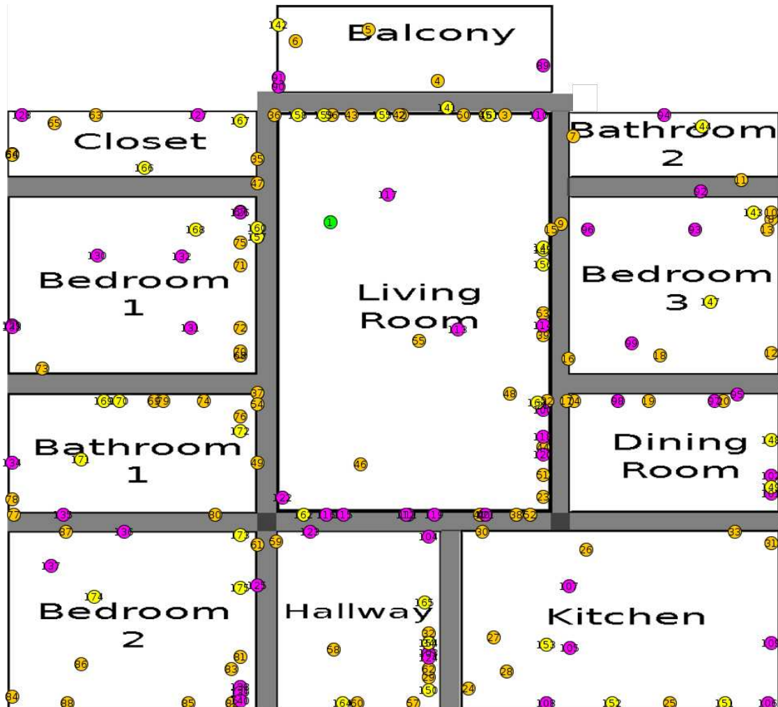
Figure 12: An example topology with 175 nodes. The green node (ID 1) is the controller, monitoring sensors are represented with orange, actuators with purple, and event sensors with yellow color.
