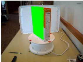
Figure 5: Planar object pose estimation using DARP.
