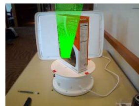
Figure 3: Planar object pose estimation using ORB.
