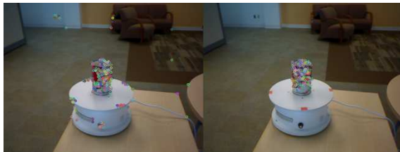
Figure 6: Non-planar object keypoint matching using ORB finds 0 matches.
